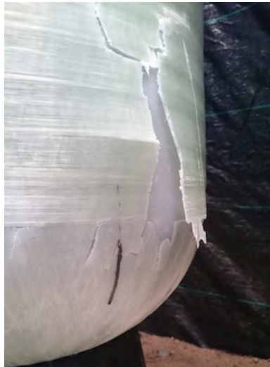
3. Implosion Tank - Partial Colapse & Broken Fiber Negative Pressure caused by siphon. No Vacuum Breaker installed. Polyethylene inner shell damaged and Fiber completely broken.
