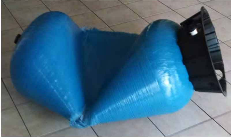
1. Implosion Tank - Total Colapse Negative Pressure caused by siphon. No Vacuum Breaker installed.
