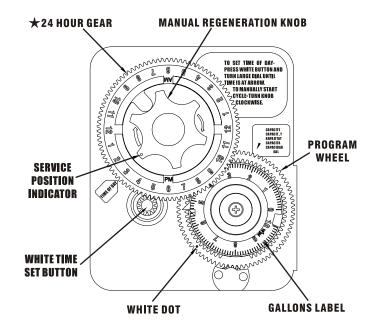
NOTE: To set meter capacity rotate manual knob 1-360° revolution to set the gallons.
